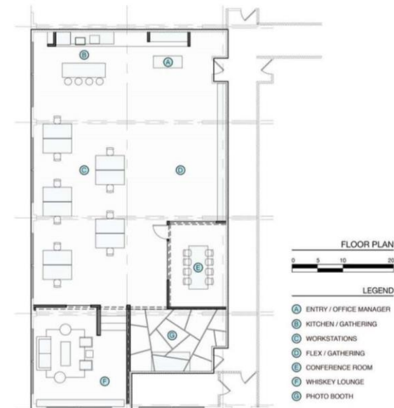
Fig.9: Plan of BeFunky office space, https://www.archdaily.com/771673/befunky-portland-office-fieldwork-design-and-architecture?ad_source=search&ad_medium=projects_tab
